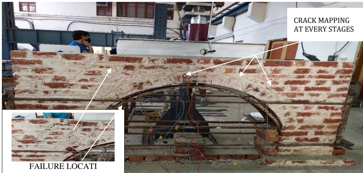
Figure 9. Failure of the structure
