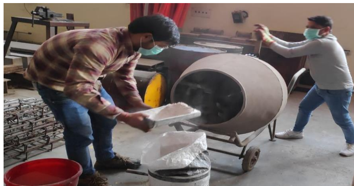
Figure 2. Mixing of lime mortar by tilting type hand mixture
