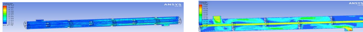
Fig 1.1(c, d): Velocity contours at the centre of shell side heat exchanger STHX-DB elliptical tube & STHX-SB elliptical tube
