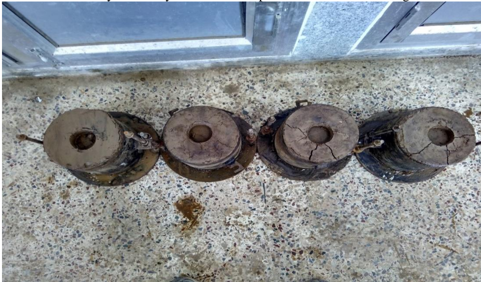
Figure 1. Tested CBR samples with and without geotextile layer
